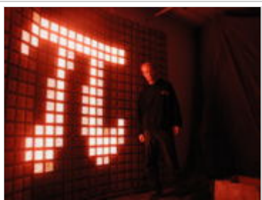
LED panels allow for smaller sets of interchangeable LEDs to be one large display.
